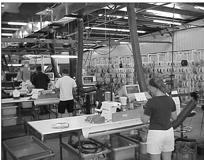
Cindy Kosch, Gary Vervoren and Cliff Sandberg are using benchtop cutting and stripping machines which allow US to produce wire harnesses efficiently.
